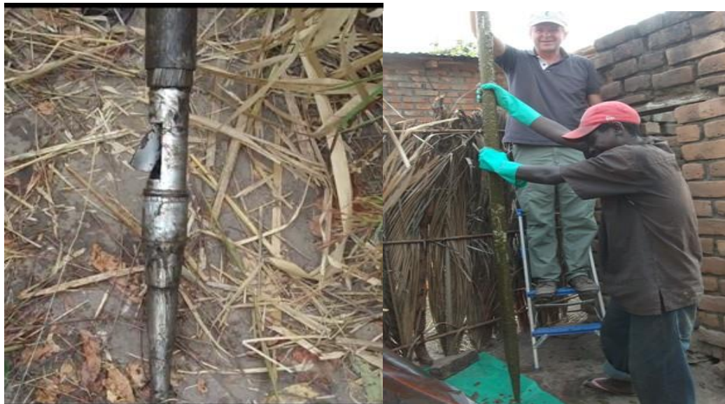
Figure 3: The standard auger used to collect the faecal samples from the pit latrines in Tanzania and Vietnam (Torondel, et al., 2016).
