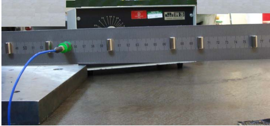
Fig. 3. The attached masses (magnets) at random locations. In total 12 masses, each weighting 2g, are used. and
