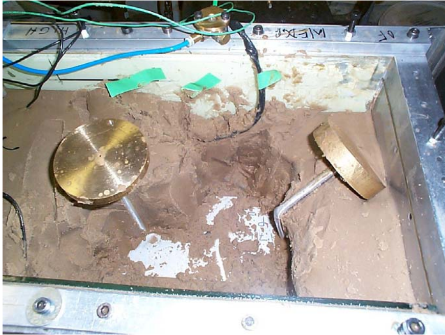
Figure 7: Piles 11 and 12 revealed during excavation in test SB-06
