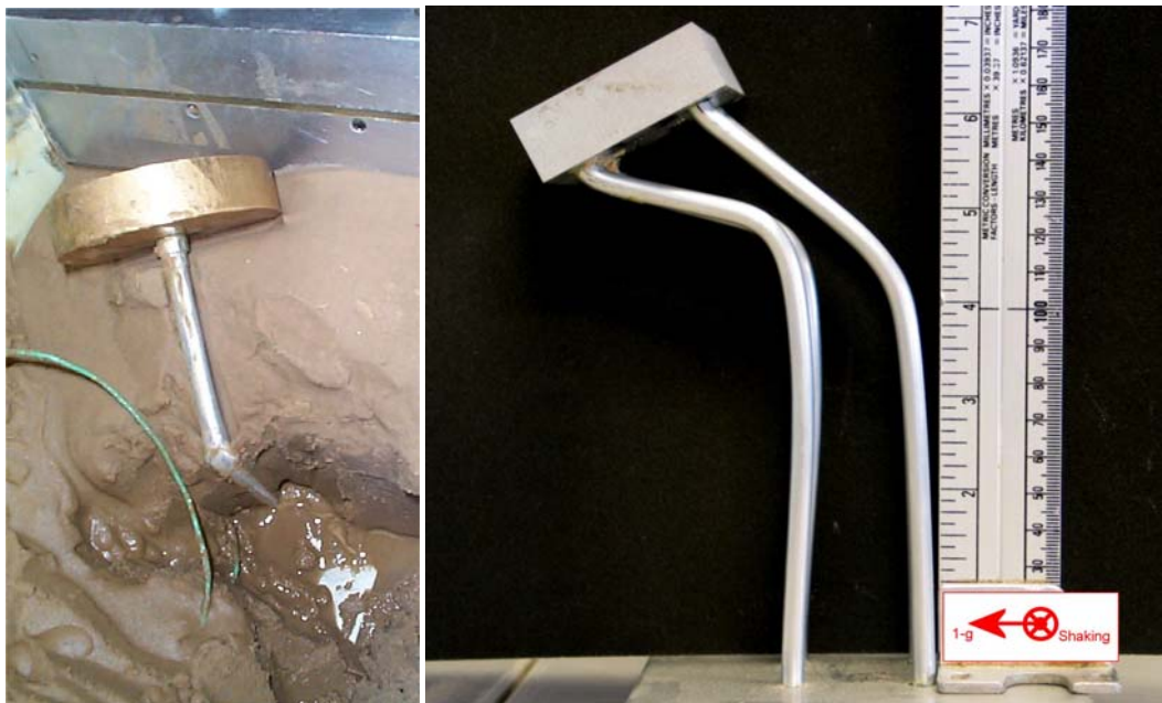
Figure 4: Instability of piled foundations observed in centrifuge tests; (a) A single pile; (b) A pile group, Knappett and Madabhushi (2005).
