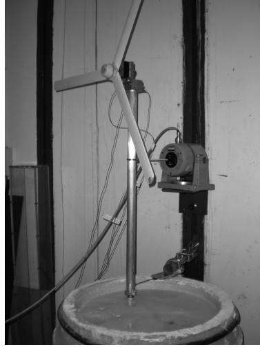
Fig. 10 The model wind turbine embedded in clay. The properties are -EI (Tower): 2.125 \times 10^9 \text{ Nmm}^2 ; EI (Pile): 3.18 \times 10^8 \text{ Nmm}^2 ; Length of the tower: 1.0 m; Length of the pile (in the clay): 0.5 m
