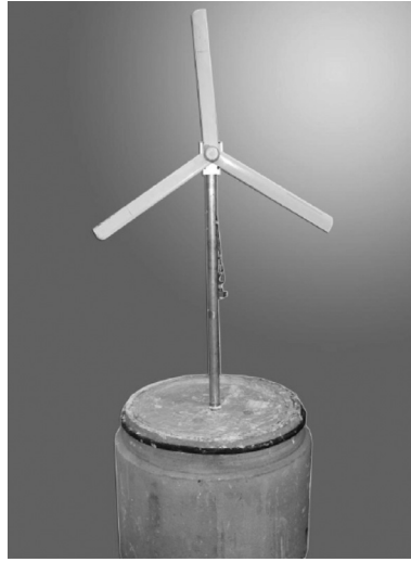
Fig. 11. The model wind turbine. The properties are - EI (Tower): 2.125 \times 10^9 Nmm 2 ; EI (Pile): 3.18 \times 10^8 Nmm 2 ; Length of the tower: 1.0 m; Length of the pile: 0.5 m.
