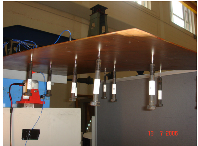
Fig. 16. Attached oscillators at random locations. The spring stiffness varies so that the oscillator frequencies are between 43 and 70 Hz.
