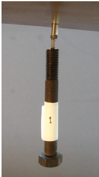
Fig. 15. Details of a typical oscillator used to simulate unmodelled dynamics. Fixed mass (magnet) 2 g, oscillatory mass (the bolt) 121.4 g. The oscillatory mass is about 1% of the total mass of the plate. The spring stiffness varies between 1.5 and 2.4 \times 10^4 N/m.
