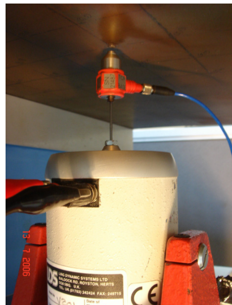
Fig. 17. The shaker used to provide an impulse excitation using Simulink™ and dSpace™. A hard steel tip was used and the shaker was placed at node (4, 6).
