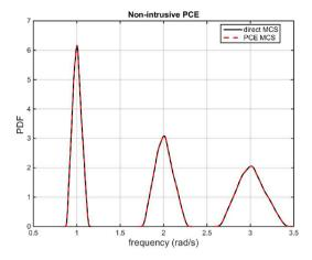
Fig. 3. Case 1: estimation of the Probability density function of the eigenfrequencies: MCS (solid black line) versus intrusive and non-intrusive PCE (dashed red line) for 2 uncertain parameters.
