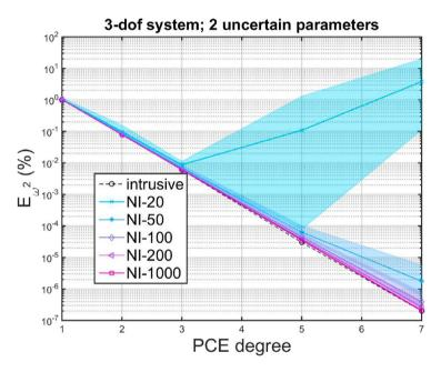
Fig. 4. 3-dof system with 2 random parameters:  $\mathcal{E}_{\omega^2}$  comparison - dashed black line: I-PCE; solid coloured lines with markers: mean of OLS-PCE errors; coloured area: envelope of NI-PCE errors.
