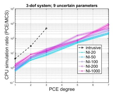
Fig. 5. 3-dof system with 9 random parameters: CPU simulation time comparison.
