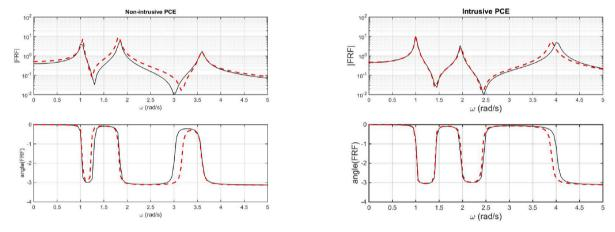
Fig. 9. Magnitude and argument of the FRF for the "worst sample" of the magnitude obtained from a direct simulation (MCS: black solid line) and the PCE of degree 3 (red dashed line); for NI-PCE,  $N_{spl} = 200$ .
