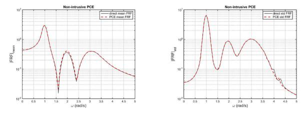
Fig. 10. Mean and standard deviation of the FRF from a direct simulation (MCS: black solid line) and NI-PCE of degree 3,  $N_{spl} = 200$  (red dashed line).
