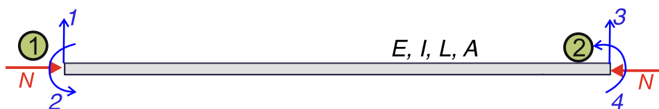
Fig. 2. An Euler–Bernoulli beam subjected to an axial force N .
