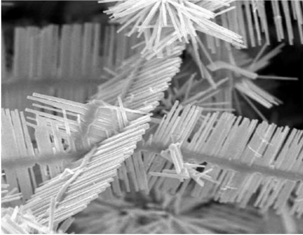
Fig. 1. ZnO side nanorods growing on central nanowire cores (Wen et al., 2003) – Physical model.
