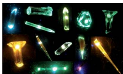
Deep-center luminescence of various ZnO samples (taken from the Review Article by C. Klingshirn, ZnO: From basics towards applications [8]).
