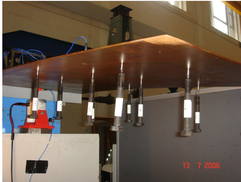
Figure 6: The test rig for the cantilever beam plate with attached oscillators at random locations.
