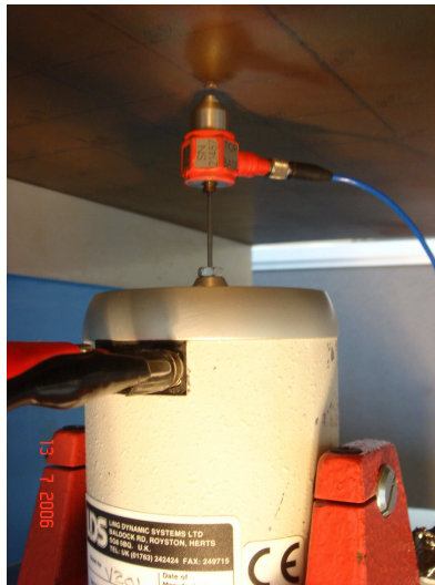
Figure 8: The shaker used to provide an impulse excitation. A hard steel tip was used and the shaker was placed at node (4,6).
