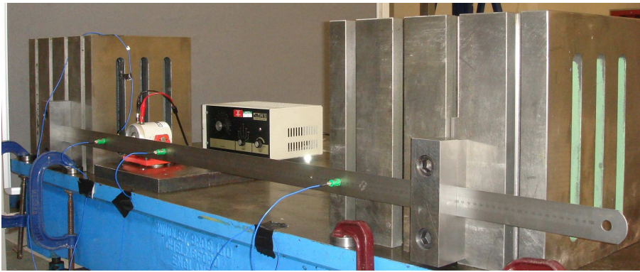
Figure 1: The test rig for the fixed-fixed beam.
