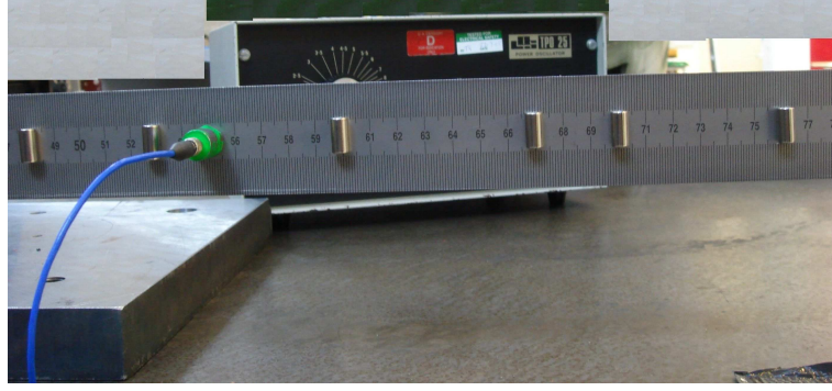
Figure 2: Attached masses (magnets) at random locations. In total 12 masses, each weighting 2g, are used.
