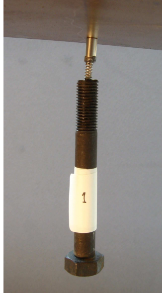
Figure 7: Details of a typical oscillator used to simulate unmodelled dynamics. Fixed mass (magnet) 2g, oscillatory mass (the nut) 121.4g. The spring stiffness varies between 15 and 24 kN/m.
