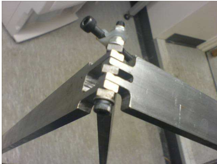
Figure 7. The three-way interleaved pin-joint at the corner of the cross-braced rectangle
