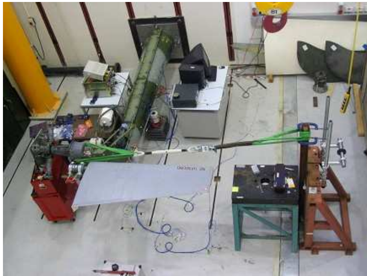
Figure 1. The lateral turnbuckle loading test setup
