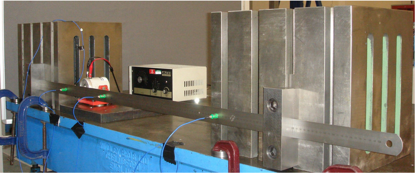
Figure 1: Experimental Setup for the Fixed-Fixed Beam
