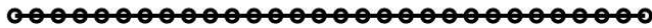
Figure 6: Schematic representation of the Finite element mesh of the of the free-free beam shown in figure 5.
