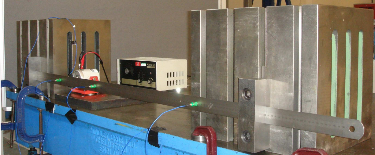
Figure 1: The test rig for the fixed-fixed beam.
