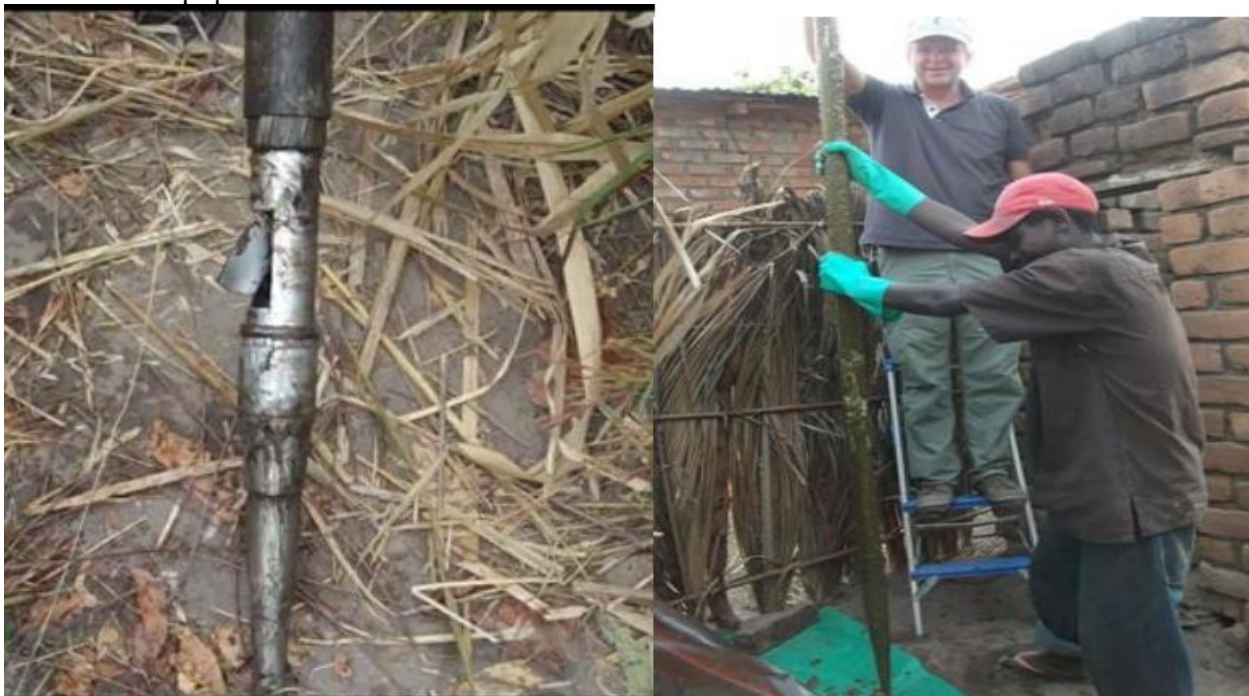
Figure 2: The standard auger used to collect the faecal samples from the pit latrines in Tanzania and Vietnam (Torondel, et al., 2016).
