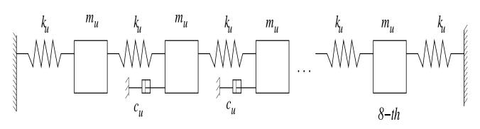
Linear array of 8 spring-mass oscillators; nominal system:  $m_u = 1$  Kg,  $k_u = 10$  N/m and  $c_u = 0.1$  Nm/s
