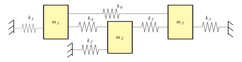
$\overline{m}_i = 1.0$  kg for i = 1, 2, 3;  $\overline{k}_i = 1.0$  N/m for  $i = 1, \cdots, 5$  and  $k_6 = 3.0$  N/m
