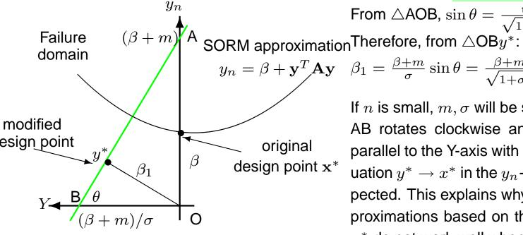
Failure surface:  $y_n - U \ge \beta$ . Using the standardizing transformation  $Y = (U - m)/\sigma$ , modified
