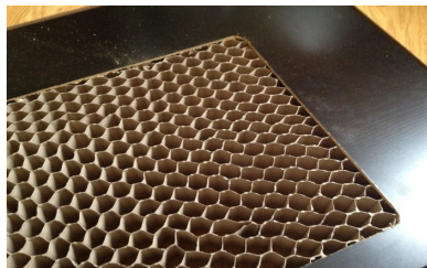
(h) Manufactured honeycomb core
