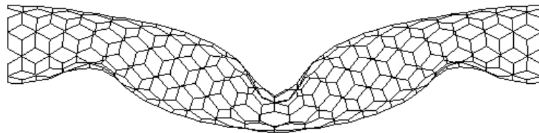
(b) Hyperelastic atomistic FE (Ogden strain energy density function)
