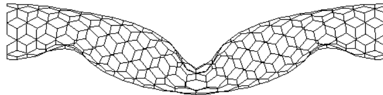
(b) Hyperplastic atomistic FE (Ogden strain energy density function)
