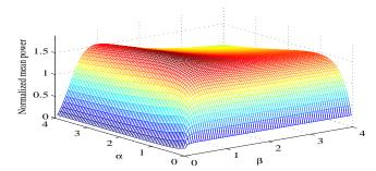
The normalized mean power of a harvester with an inductor as a function of  $\alpha$  and  $\beta$ , with  $\zeta=0.1$  and  $\kappa=0.6$ .
