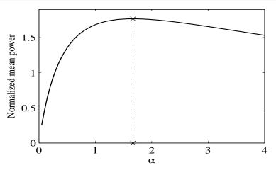
The normalized mean power of a harvester with an inductor as a function of  $\alpha$  for  $\beta=1$ ,  $\zeta=0.1$  and  $\kappa=0.6$ . The \* corresponds to the optimal value of  $\alpha(=1.667)$  for the maximum mean harvested power.
