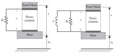
Schematic diagrams of piezoelectric energy harvesters with two different harvesting circuits. (a) Harvesting circuit without an inductor, (b) Harvesting circuit with an inductor.
