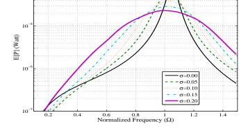
The mean power for various values of standard deviation in natural frequency with  $\bar{\omega}_n = 670.5\,\mathrm{rad/s}, \Psi_{\zeta} = 1, \alpha = 0.8649, \kappa^2 = 0.1185.$
