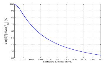
The mean harvested power for various values of standard deviation of the natural frequency, normalised by the deterministic power ( $\bar{\omega}_n = 670.5 \, \mathrm{rad/s}$ ,  $\Psi_\zeta = 1$ ,  $\alpha = 0.8649$ ,  $\kappa^2 = 0.1185$ ).
