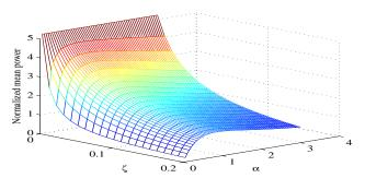
The normalized mean power of a harvester without an inductor as a function of  $\alpha$  and  $\zeta$ , with  $\kappa=0.6$ . Maximizing the average power with respect to  $\alpha$  gives the condition  $\alpha^2 \left(1+\kappa^2\right)=1$  or in terms of physical quantities  $R_r^2 C_n \left(kC_n+\theta^2\right)=m$ .
