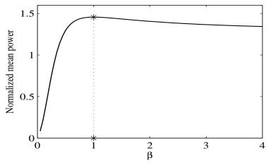
The normalized mean power of a harvester with an inductor as a function of  $\beta$  for  $\alpha = 0.6$ ,  $\zeta = 0.1$  and  $\kappa = 0.6$ . The \* corresponds to the optimal value of  $\beta (= 1)$  for the maximum mean harvested power.
