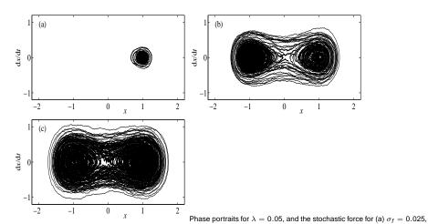
(b)  $\sigma_f = 0.045$ , (c)  $\sigma_f = 0.065$ . Note that the increasing noise level overcomes the potential barrier resulting in a significant increase in the displacement x.
