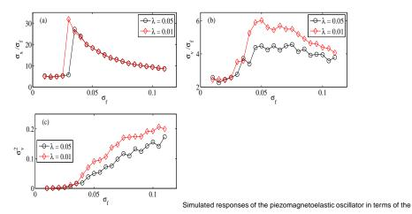
standard deviations of displacement and voltage ( $\sigma_x$  and  $\sigma_v$ ) as the standard deviation of the random excitation  $\sigma_f$  varies. (a) gives the ratio of the displacement and excitation; (b) gives the ratio of the voltage and excitation; and (c) shows the variance of the voltage, which is proportional to the mean power.
