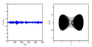
Voltage output due to Gaussian white noise ( $\zeta = 0.01$ ,  $\chi = 0.05$ , and  $\kappa = 0.5$  and  $\lambda = 0.01$ .
