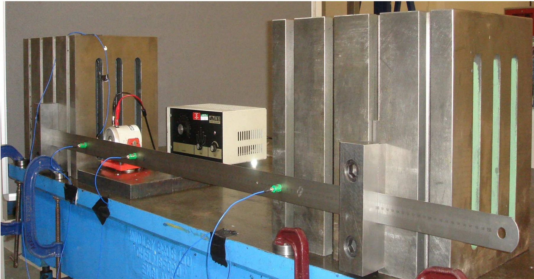
A fixed-fixed beam: Length: 1200 mm, Width: 40.06 mm, Thickness: 2.05 mm, Density: 7800 kg/m 3 , Young's Modulus: 200 GPa
