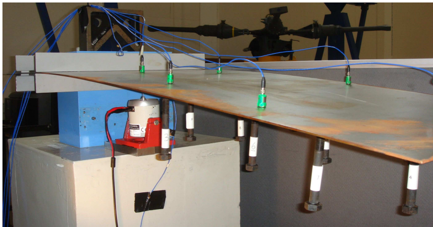
The test rig for the cantilever plate; front view.
