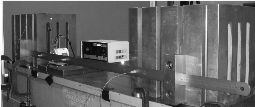
Fig. 1 Test rig for the fixed-fixed beam.
