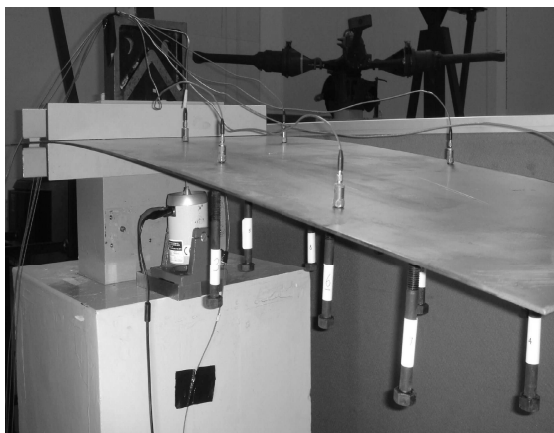
a) Experimental setup showing the accelerometer locations
