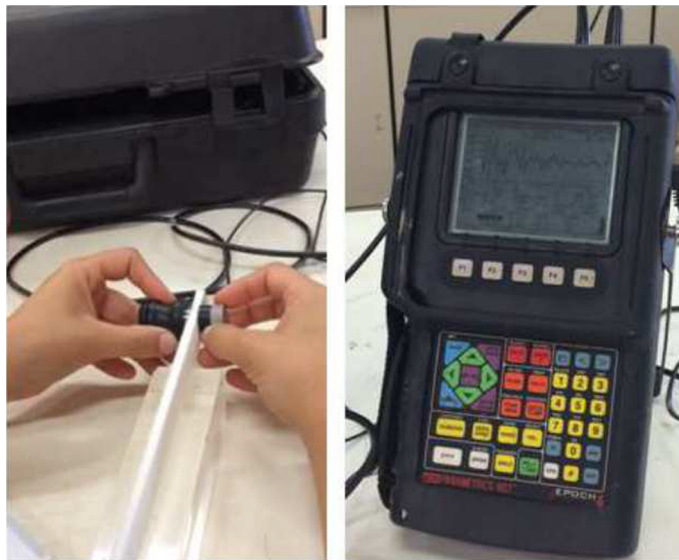
Fig. 17. Procedure for experimental measurement of polyamide beam properties.
