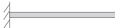
Fig. 1. Euler–Bernoulli beam with spatially varying random bending rigidity w(x, \theta) . The length of the beam is L = 1.65 \text{ m} , the section area is A = 8.2123e - 5 \text{ m}^2 , the density is \rho = 7800 \text{ kg/m}^3 and the mean of the bending rigidity random field is E[w(x, \theta)] = 5.7520 \text{ kg.m}^2 .
