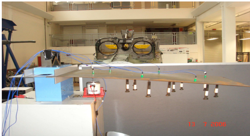
The test rig for the cantilever plate; side view.
