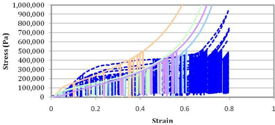
**Figure 2.** Compressive stress strain graph for PU foam. - - - PU foam blocks, \_\_\_\_\_ PU foamed layers.
