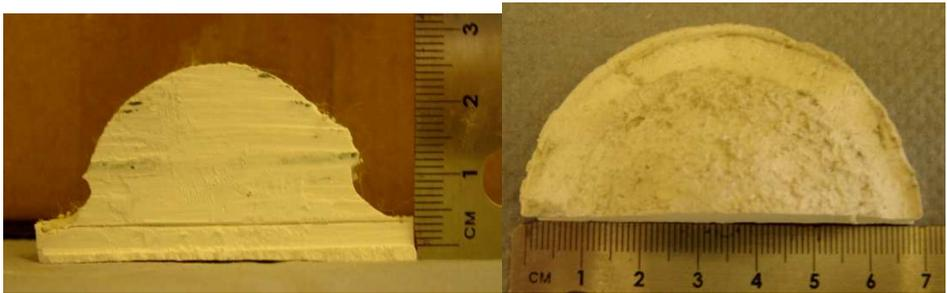
**Figure 15,** BFS molds made from plaster.
