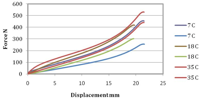
Figure 6, Force/displacement graph of clay backing, strain rate 1000mm/min.
