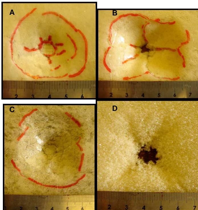
**Figure 18,** The impact face of four trauma packs. A) 3 ply foamed layers with srPP. B) 3 ply foamed layers with no srPP. C) 4 ply foamed layers with srPP. D) 3 ply sliced layers no srPP.
