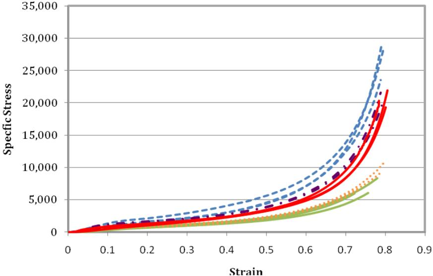
**Figure 5.** Specific stress strain graph for trauma pack samples. --- 3 foamed layers, --- 3 foamed layers flexible, — foamed layers no srPP, ..... 4 foamed layers flexible, — 4 foamed layers flexible
