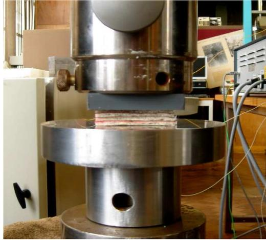
**Figure 1.** Foamed layers under compression.
