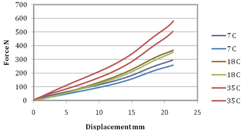
Figure 8, Force/displacement graph of clay backing, strain rate 10,000mm/min.
