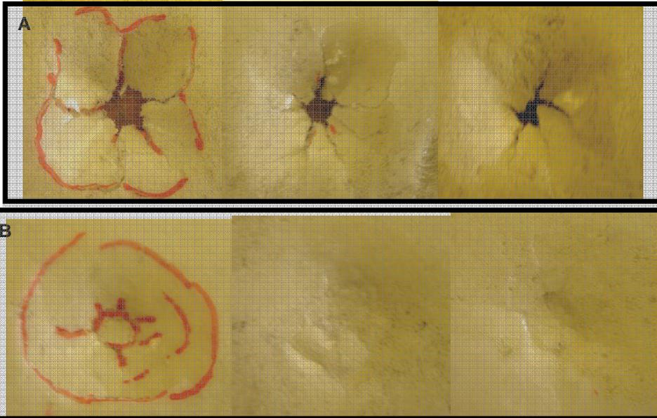
**Figure 19,** The progression of deformation through two trauma packs, A) Foamed layers without srPP, B) Foamed layers with srPP.
