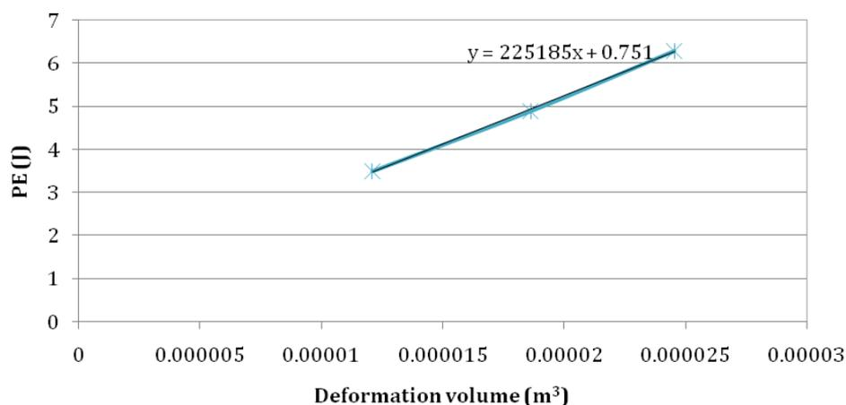
**Figure 9,** Potential energy / deformation volume graph for drop tests on clay backing.
