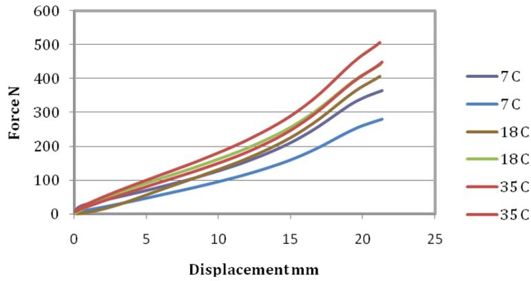
Figure 7, Force/displacement graph of clay backing, strain rate 5000mm/min.
