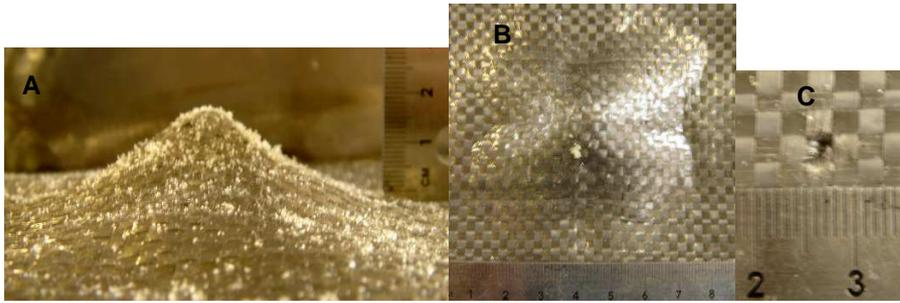
**Figure 11**, srPP armor after ballistic test. A) BFS side view, B) BFS top view, C) Entry hole on impact face.
