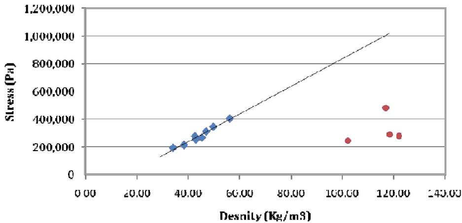
**Figure 3.** Compressive stress at 40% strain against specimen density, ◆ Foam blocks, ● Foamed Layers.
