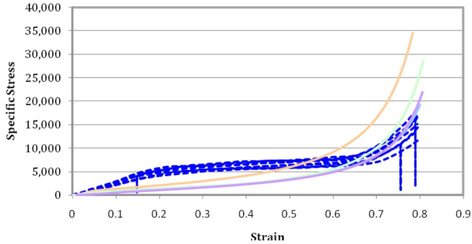
**Figure 4.** Specific stress strain graph for PU foam. - - - PU foam blocks, \_\_\_\_\_ PU foamed layers.
