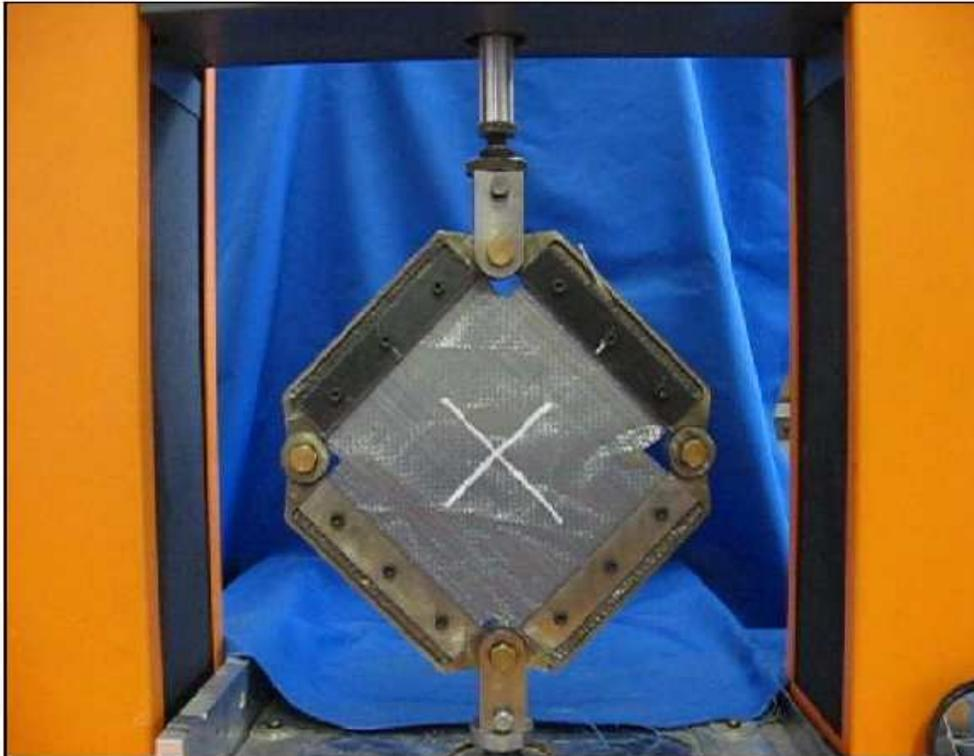
Figure 11 shows the experimental setup for the picture frame test in which sample was clamped tightly.
