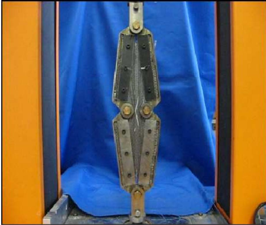
Figure 12a shows fully extended picture frame rig and deformed tightly clamped sample.
