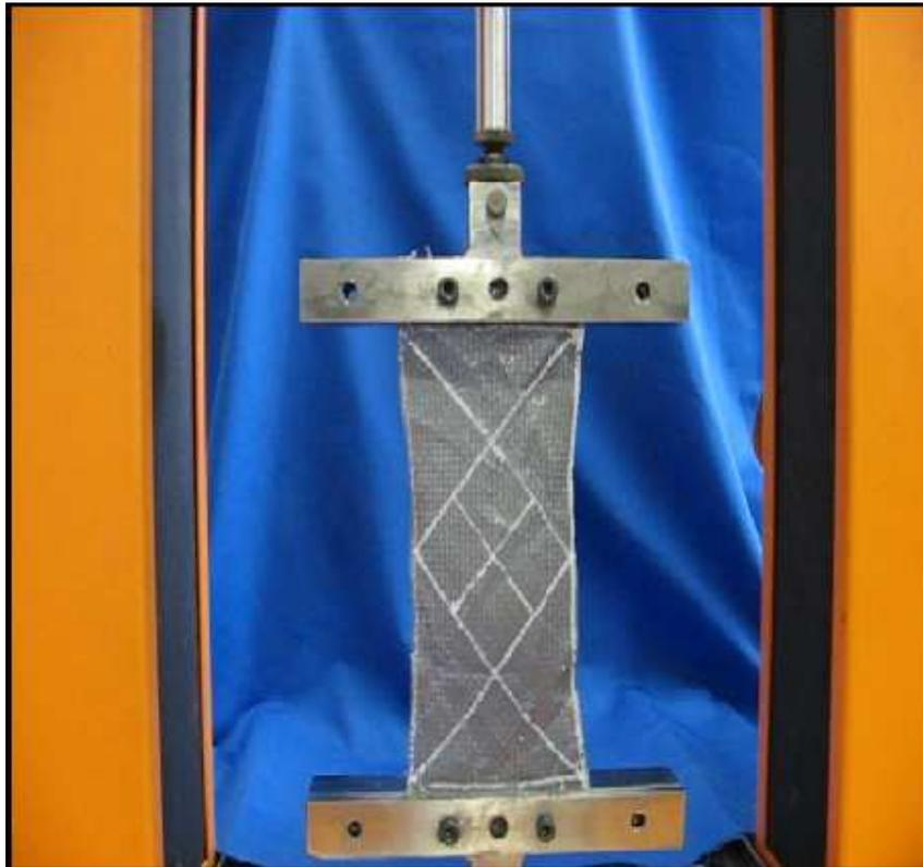
Figure 14 shows experimental setup for bias extension test and a prepared sample clamped in it.
