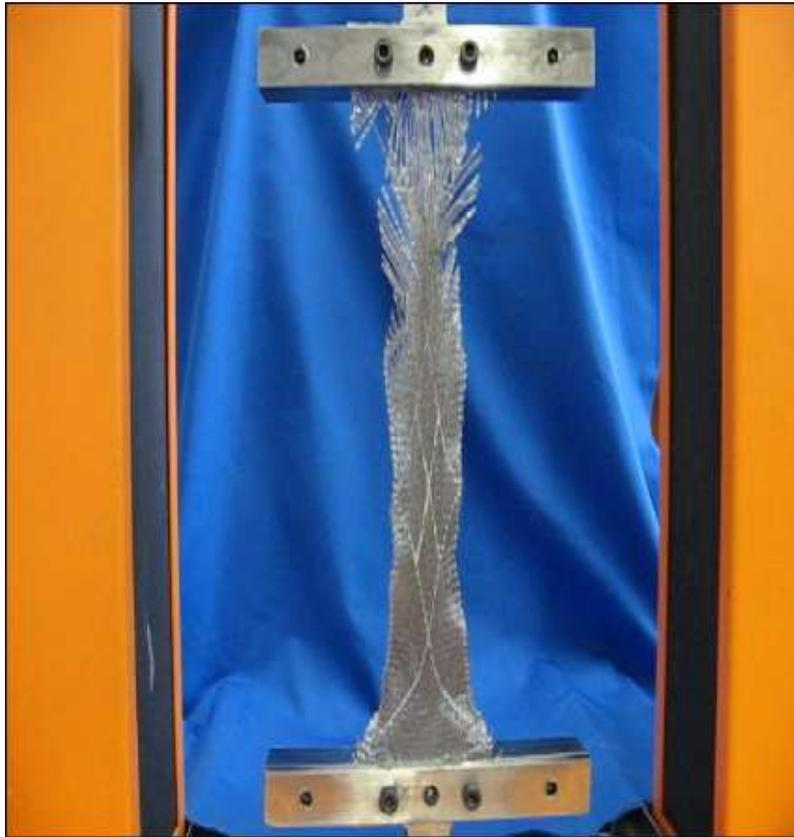
Figure 15 shows destructive deformation of the composite sample.
