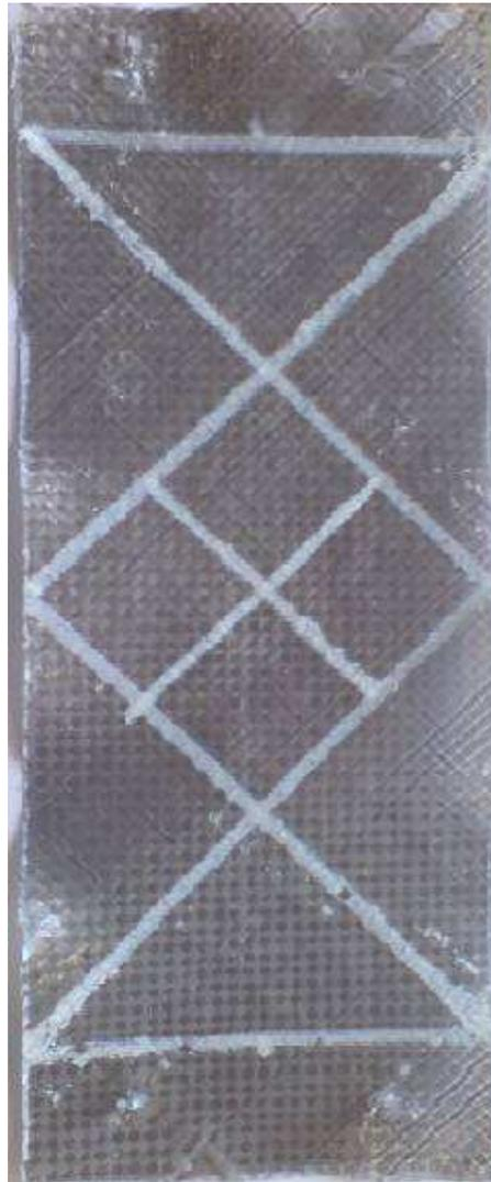
Figure 13 shows prepared sample for bias extension test with marking on it.
