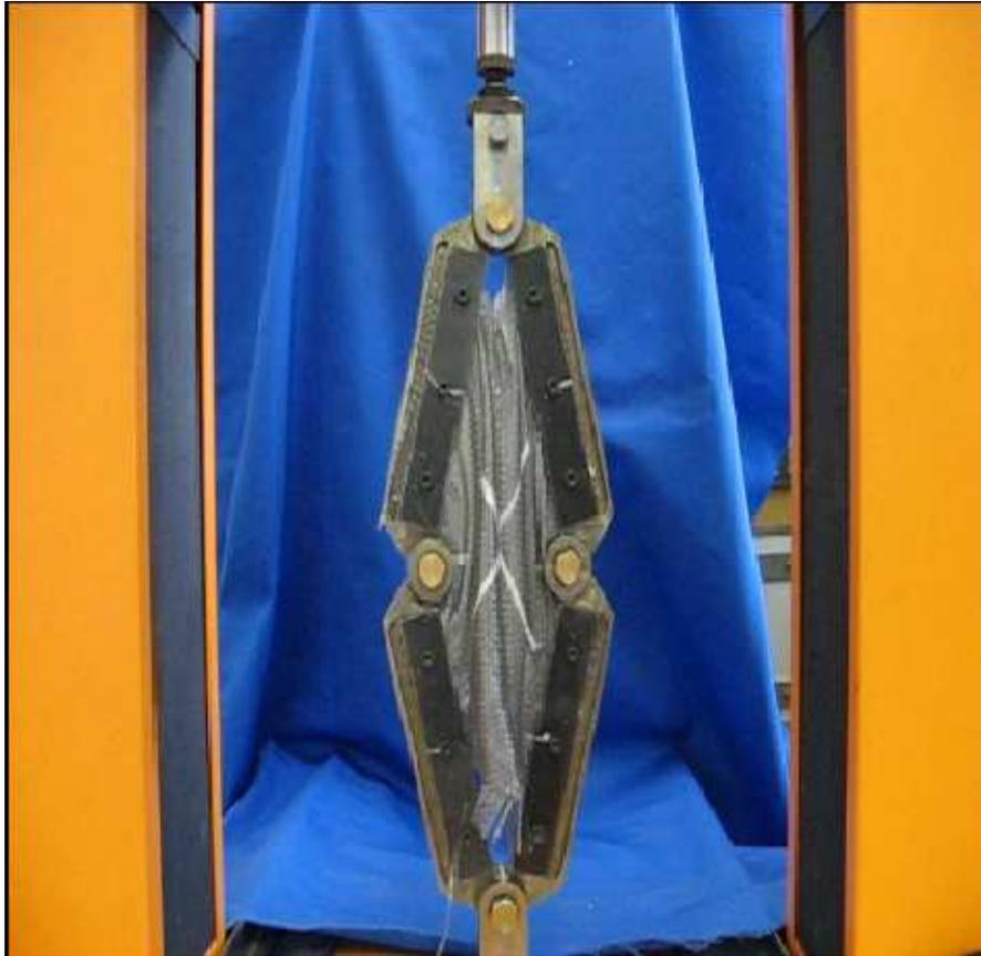
Figure 12b shows the fully extended picture frame and deformed loosely clamped sample.
