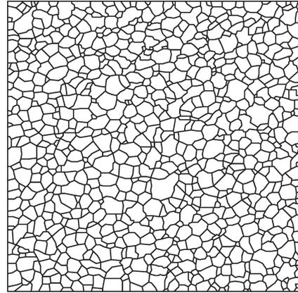
Fig. 3. Image of grain boundaries extracted from an AFM image of polysilicon grains.
