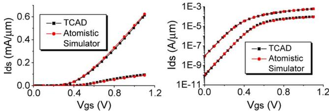
Fig. 2. Calibration of "atomistic" simulator on nominal-device TCAD data.
