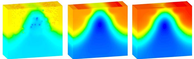
Fig. 4. Typical potential distributions corresponding to individual IPF source. From left to right, illustrations show the effect of RDD, LER, and PGG.
