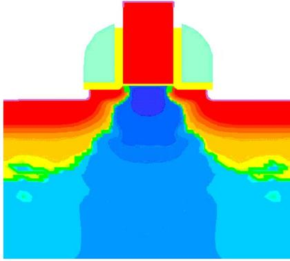
Fig. 1. Nominal-device structure and net-doping profile.
