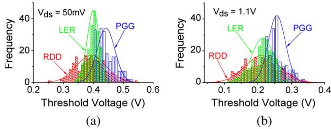
Fig. 5. Threshold-voltage distribution due to RDD, LER, and PGG. (a)  $V_{ds} = 50$  mV. (b)  $V_{ds} = 1.1$  V, while for PGG, the Fermi pinning potential is 200 mV above midgap.
